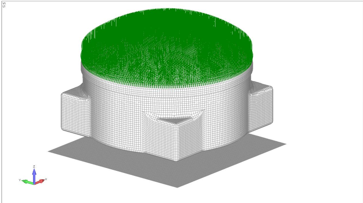
*Figure 4-6. Definition of distributed loading for hatch of access chamber.*
