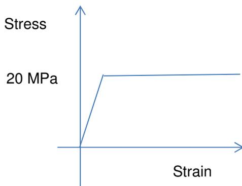
*Figure 4-1. Assumed stress strain curve for polyethylene.*
