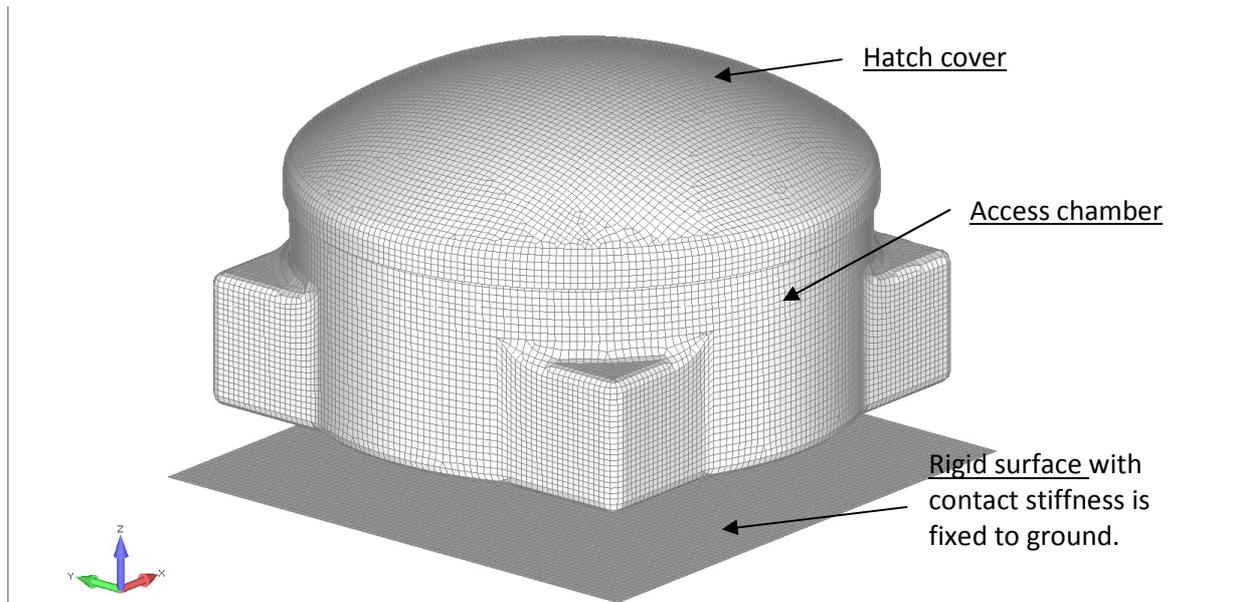
*Figure 4-2. Global model of the access chamber*
