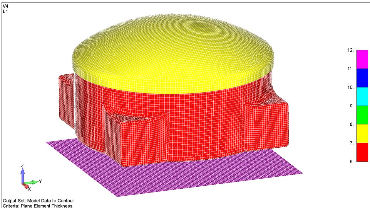
Figure 4-4. Wall thickness for hatch cover and access chamber.
