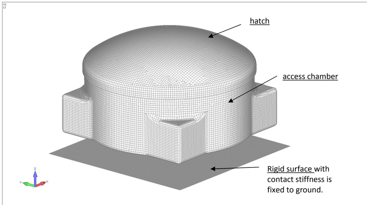
Figure 4-5. Boundary conditions for turret structure.
